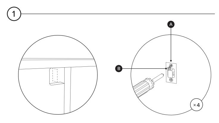
Attach bracket to each inside edge approx. 1.5" in through the holes on the back of the headboard. Note there are no existing pilot holes on the product.
